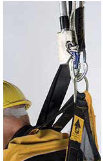
Rescue pole being used to connect to hook on rear of harness.
