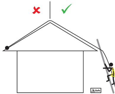
**Climb ladder moving adjuster as you climb to minimise free fall before the shock absorber would be deployed**
