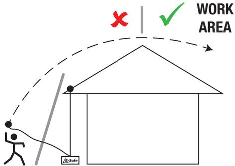
**Test connection, move adjuster to knot end and throw to opposite side**
