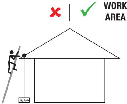
**Set ladder and establish Anchor then Connect Rope Line**
