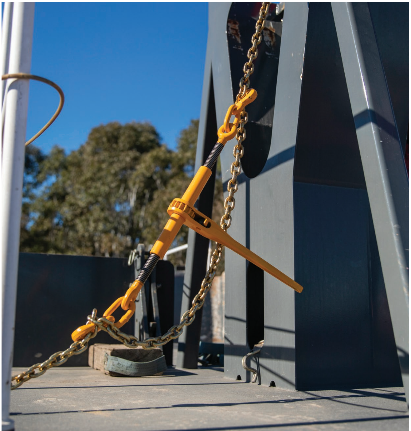
The handle of the BX600 moves freely to the beginning of the release point.
